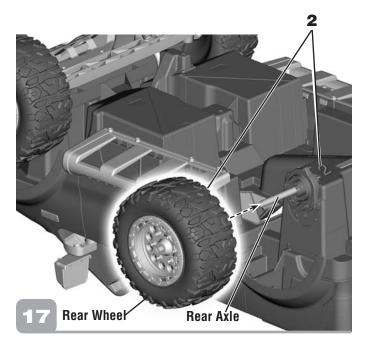
•Slide a rear wheel onto the rear axle.
